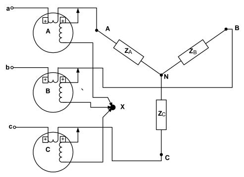
Figure 2 Three watt meters connected to monitor power taken by a three-phase load.
