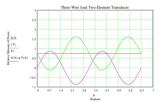
Graph Set 5 - 0 Power Factor. No power is used by the load even though it is drawing current and is supplied with voltage.
